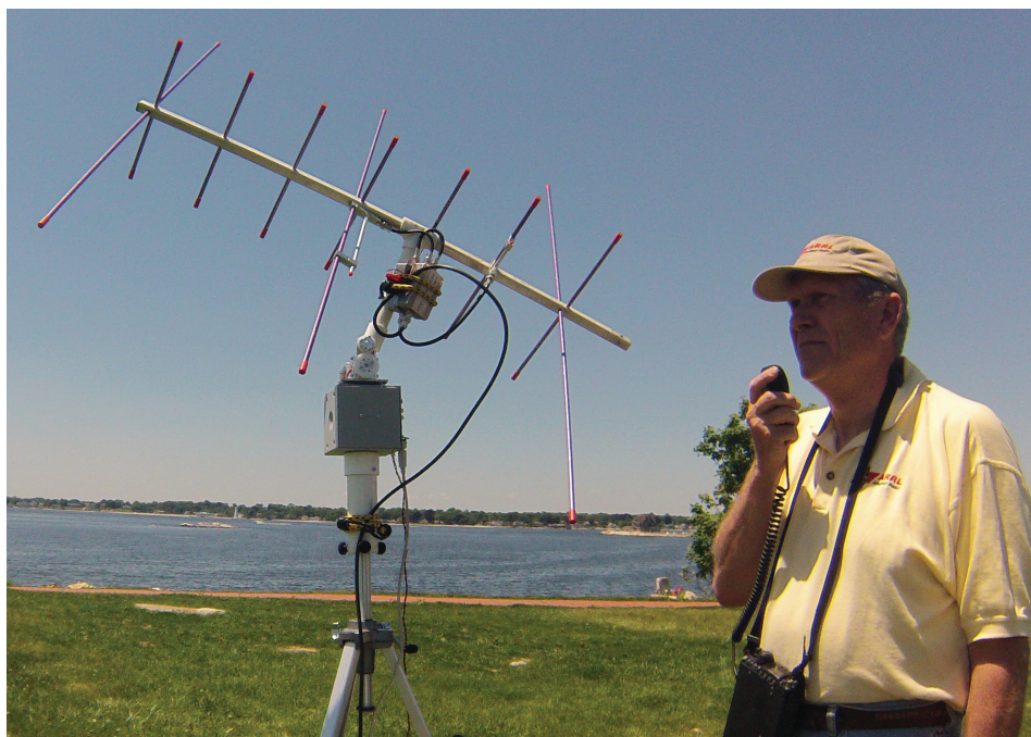
The author shown with his original WRAPS rotator project described in the January 2014 QST . This article shows how to add the capability to modify WRAPS with two beams and add the capability for circular polarization.
